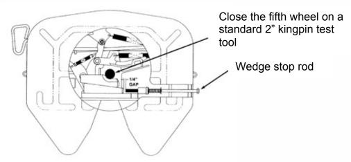
Figure 3: Image of the test kingpin and the wedge stop rod
