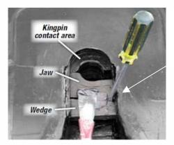
Separate the jaw and wedge with the screw driver here – grease the full length
