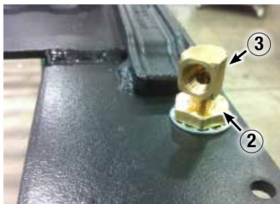
Figure 3: 90° street elbow screwed into bulkhead fitting
