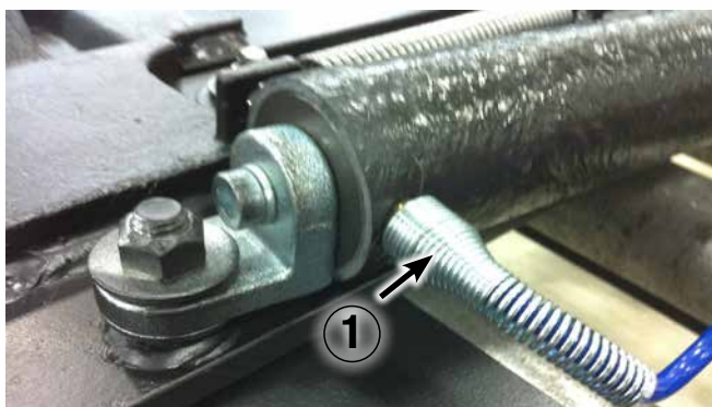
Figure 6: Air line coil screwed into air cylinder
