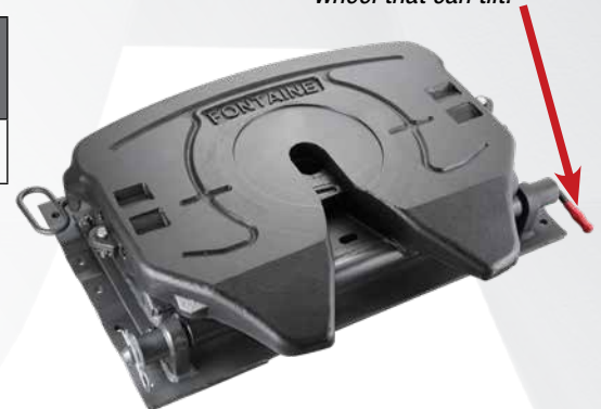
Removing blocking bar converts "No-Tilt" blocked fifth wheel to standard fifth wheel that can tilt.
