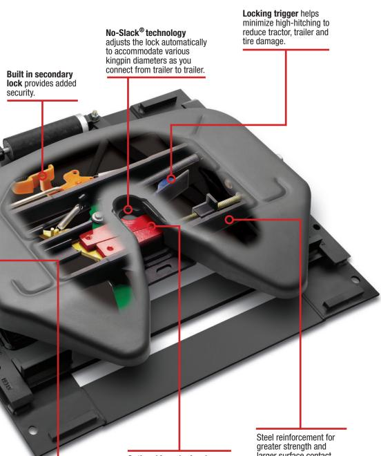
Easiest straight pull handle in the industry. Just pull the handle to open the lockno complicated opening sequence to remember.
