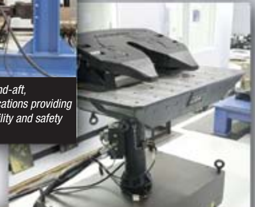
Single Axis Shaker Table applies vibration profiles to fifth wheel components. Information gathered here helps us improve durability for lock components, sensors, air cylinders, and auto lube components.
