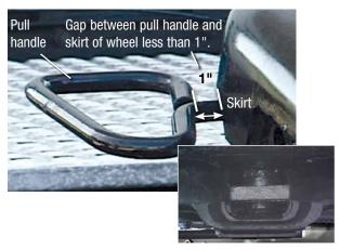
Use a flashlight and go under the trailer and look into the back of the throat of the fifth wheel. The locking mechanism should be engaged across the entire throat of the fifth wheel and secured to the kingpin.
