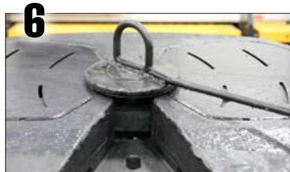
Tilt the fifth wheel down and lower the yard truck boom.
