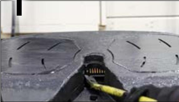
Trip the wheel closed using a crowbar. **NEVER use hands to trip an activated fifth wheel.**
