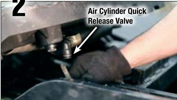
Raise the yard truck boom for easy access, then remove the air hose from the air cylinder quick release valve.
