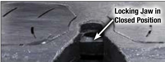
**Hint:** A fifth wheel is closed when the locking jaw is completely across the throat of the fifth wheel.
