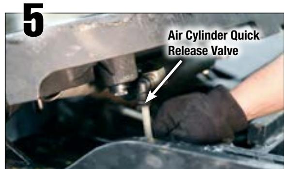
Connect the air hose to the air cylinder quick release valve.
