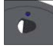
Air cylinder bolt access (under wear plate)
