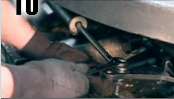
Remove air cylinder/secondary lock bolt.
